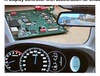
BADGE works as a graphics engine in embedded systems, but doesn't suffer from the short life cycles affecting the usual graphics controllers. It is very flexible. Can interface to numerous types of processors, memories and displays.
